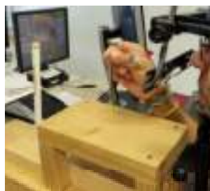
Figure 1: Experimental set up for the bead threading task using two infrared markers and eye-tracker.
