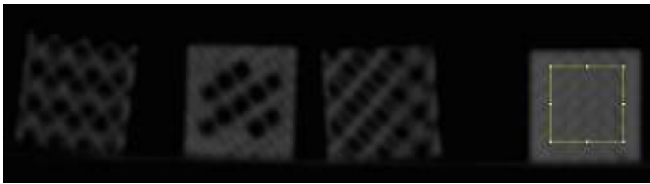
Fig. 3. An axial slice of the scanned cubes showing a selected ROI (yellow square) for one of the cubes. The same ROI size and positioning were consistently applied across twenty consecutive slices of each cube.
