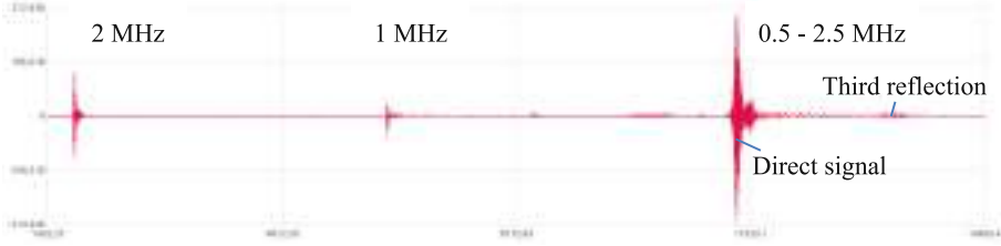
Fig. 2. Example of train of received ultrasonic signals in a single run.
