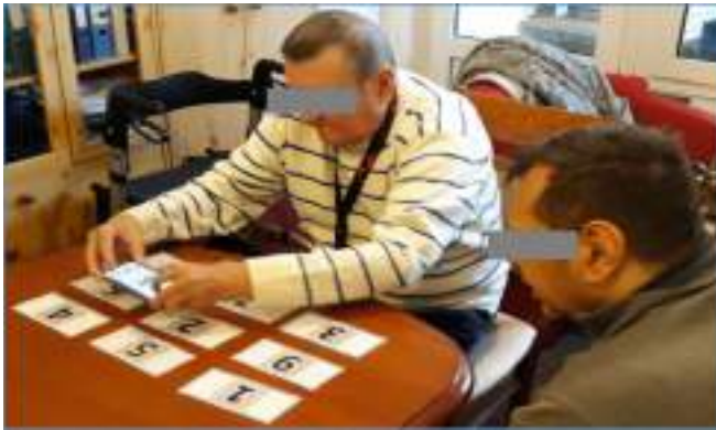
Fig. 1. An example of a game using a mobile phone with a NFC reader and NFC tags placed on cards.
